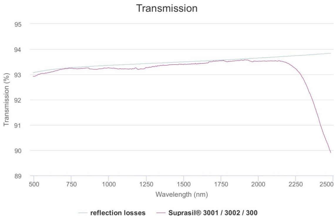
Figure 45. Transmissivity curve of a Suprasil 3002 slab having thickness 80 mm. The internal transmissivity is given by the difference between reflection loss and transmission curves.
