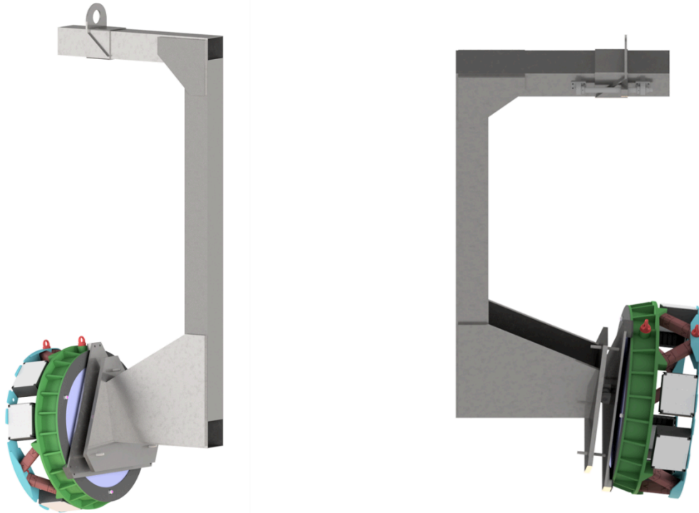
Figure 29: C-shaped handling for M9 installation. The interface between M9 and the handling is between the 3 pads at the front flange (in green) and the 3 connection pads of the handling. The handling is equipped with a hook hoisting connection point having the possibility to slide, in order to have it aligned with the barycentre of the system both when M9 is connected and disconnected.
