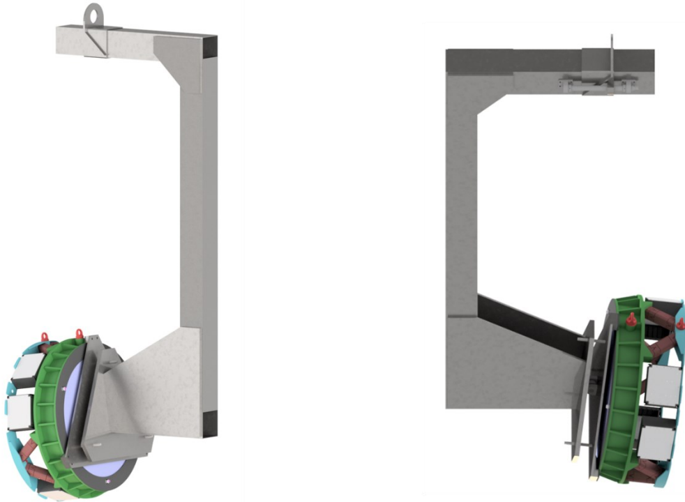
Figure 10: C-shaped handling for M9 installation. The interface between M9 and the handling is between the 3 pads at the front flange (in green) and the 3 connection pads of the handling. The handling is equipped with a hook hoisting connection point having the possibility to slide, in order to have it aligned with the barycentre of the system both when M9 is connected and disconnected.
