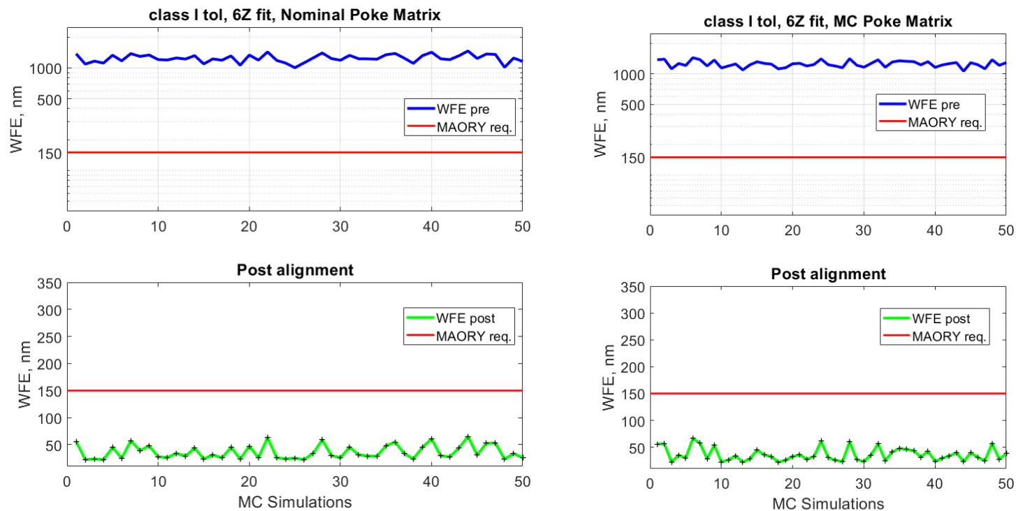
Figure 68 WFE pre alignment (top) & post (bottom) for 50 MC simulations for class I positioning tolerances corrected with a poke matrix retrieved from the nominal MAORY design (left) and for poke matrices built for each MC realization (right). In both the samples the Donuts were fitted with 6 Zernike terms.
