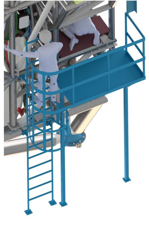
Figure 142: red scaffoldings provide a working area to 2 people and support to the protruding part of the rails.
