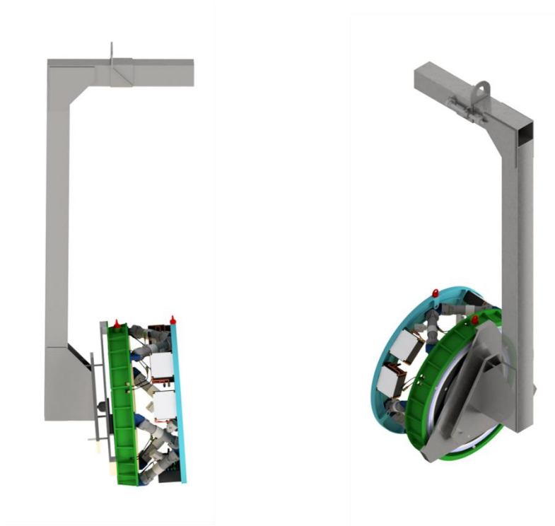
Figure 21: C-shaped handling for M10 installation. The interface between M10 and the handling is between the 3 pads at the front flange (in green) and the 3 connection pads of the handling. The handling is equipped with a hook hoisting connection point having the possibility to slide, in order to have it aligned with the barycentre of the system both when M9 is connected and disconnected.
