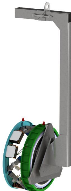
Figure 130: C-shaped handling for the installation of M10 in the MSS
