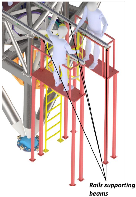
Figure 142: red scaffoldings provide a working area to 2 people and support to the protruding part of the rails.
